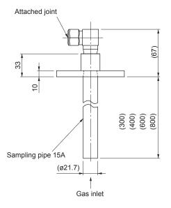
Attached joint (for ø6 pipe connection)
