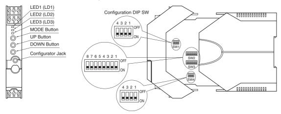
The DIP switch setting is required to select output types before setting a precise output range using the PC configurator software.
