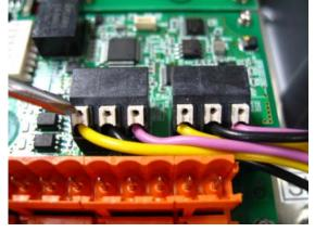
Note) Be sure to remove Path 2 connector when wiring cable from resistance bulb to temperature input board.
