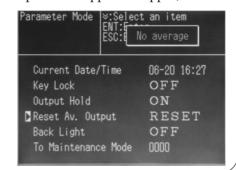
(1) Using the ( key, move the cursor to <Reset Av. Output>, and then press the (ENT) key.
