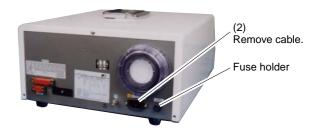
(3) Turn the cap of the fuse holder counterclockwise, and pull it toward you.
