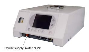
(2) The WARM-UP display comes on and stays on for about 2 seconds in the center. It then moves to the lower left-hand corner of the screen. The warm-up operation end time is displayed with the down timer.
