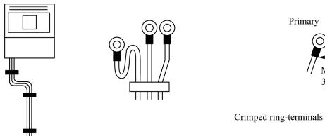
Reinforced insulation must be maintained over safe separation on termination of wires/crimps.
