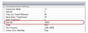
IP address, port number, and maximum read value of the PLC
