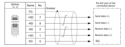
• If noise disturbs communications, connect a shielded cable to both the X1 series unit and the connected device.
