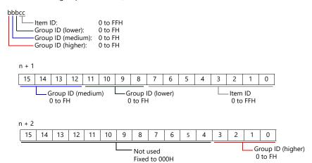
\*2 In the expansion code, specify the sub-station number, and set which word, higher or lower, is to be read when a 2-word address is specified (expansion bit designation).
