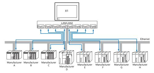
• When multiple PLCs of the same model are connected, a single port on the X1 series unit can be used to perform 1: n communication with these PLCs.
