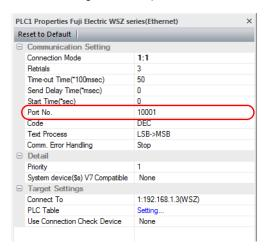
IP address, port number, and maximum read value of the PLC
