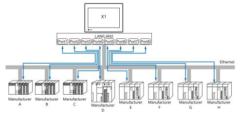
When there are two or more PLCs of the same model, the X1 series can carry out 1: n communication via one port.
