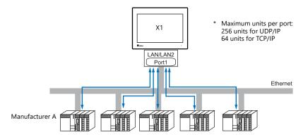
• If multiple X1 series units are connected to one single PLC, the maximum permissible number of these units depends on the PLC specifications. Refer to the PLC manual issued by the manufacturer.
