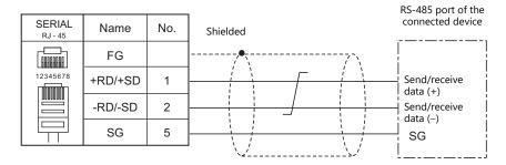
• If noise disturbs communications, connect a shielded cable to both the X1 series unit and the connected device.
