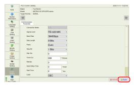
\* Press the [Restore Screen Data Settings] switch to restore the screen program settings.
