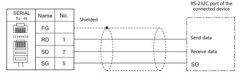
• If noise disturbs communications, connect a shielded cable to both the X1 series unit and the connected device.
