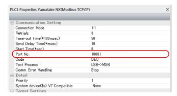
IP address, port number, and maximum read value of the PLC
