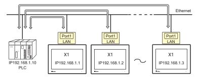
• You can make settings for Ethernet communication in [Communication Setting] for the logical ports PLC1 - PLC8.
