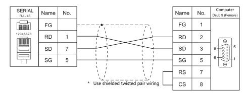
\* Select RS-232C in the screen program or on the Local mode screen of the X1 series unit. For details, see "1.2.1 SERIAL" (page 1-4).
