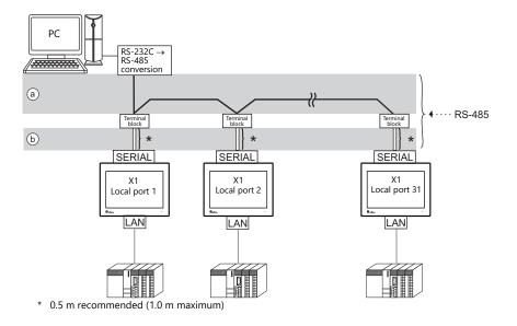
• Wiring example of above (a) and (b)
