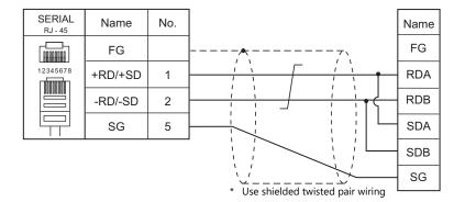
\* Select RS-422/485 in the screen program or on the Local mode screen of the X1 series unit. For details, see "1.2.1 SERIAL" (page 1-4).
