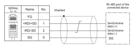
• If noise disturbs communications, connect a shielded cable to both the X1 series unit and the connected device.
