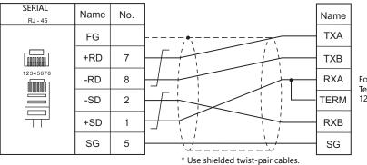
For 1 : 1 connection: Terminating resistance: 120  $\Omega$  with RXA and TERM short-circuited
