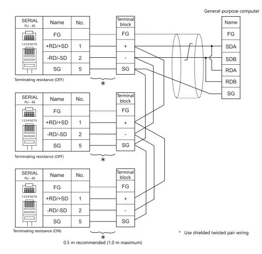
\* Select RS-422/485 in the screen program or on the Local mode screen of the X1 series unit. For details, see "1.2.1 SERIAL" (page 1-4).
