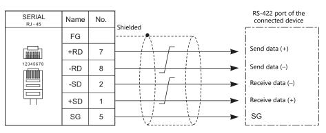
• If noise disturbs communications, connect a shielded cable to both the X1 series unit and the connected device.
