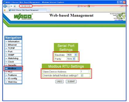
Enter the IP address of the bus coupler or bus controller on Internet Explorer, and press the [Enter] key to display the browser menu.
