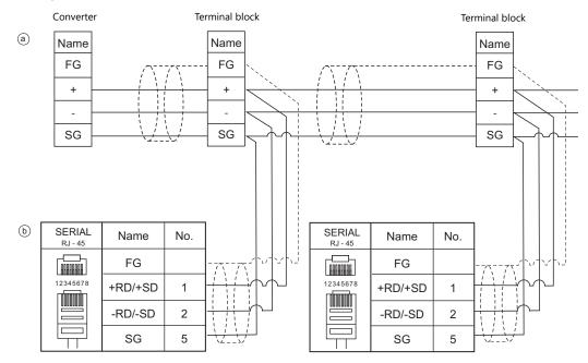
\* Select RS-422/485 in the screen program or on the Local mode screen of the X1 series unit. For details, see "1.2.1 SERIAL" (page 1-4).
