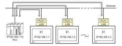
• You can make settings for Ethernet communication in [Communication Setting] for the logical ports PLC1 - PLC8.
