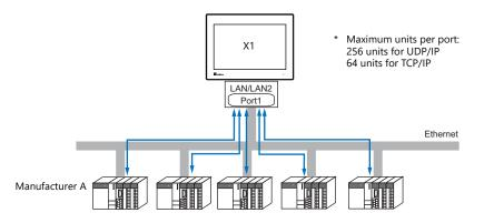
• If multiple X1 series units are connected to one single PLC, the maximum permissible number of these units depends on the PLC specifications. Refer to the PLC manual issued by the manufacturer.
