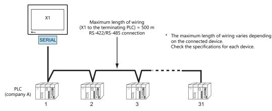
• For models that support multi-drop connection, refer to the "Connection Compatibility List" provided at the end of this manual or the chapters on individual manufacturers.
