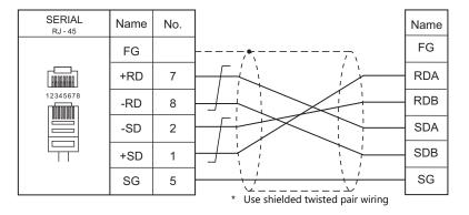
\* Select RS-422/485 in the screen program or on the Local mode screen of the X1 series unit. For details, see "1.2.1 SERIAL" (page 1-4).
