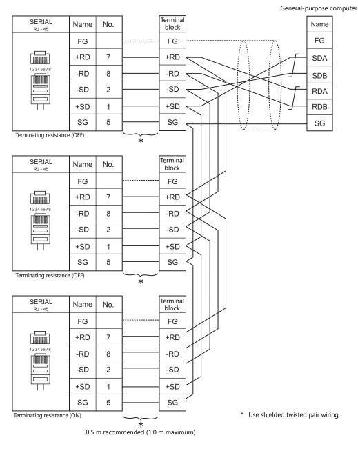
\* Select RS-422/485 in the screen program or on the Local mode screen of the X1 series unit. For details, see "1.2.1 SERIAL" (page 1-4).
