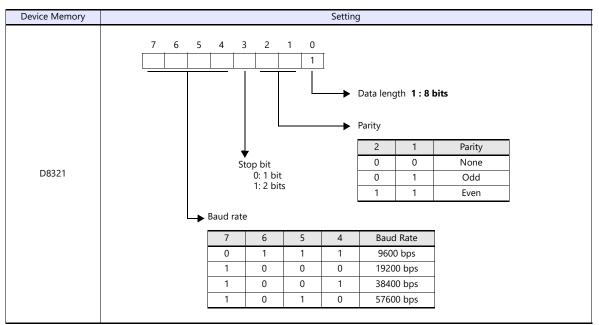
\* If the value specified for any item is outside the allowable range, the item will be assumed to be: data length: 8 bits, parity: none, stop bit: 2 bits, or baud rate: 19200 bps.
