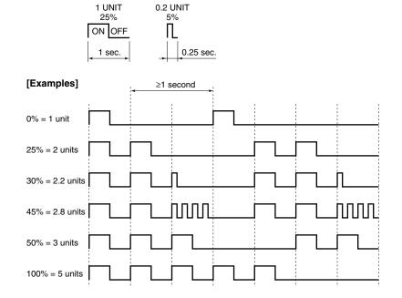
**ERROR MONITOR:** Indicates the transmitter's error status.
