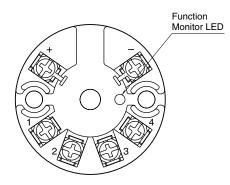
■ INPUT MONITOR: The input 0 – 100% is converted into a combination of 1-second (1 unit) and 0.25-second (0.2 unit) cycled pulses. 1 unit corresponds to 25%, while 0.2 unit corresponds to 5%. 0% equals to 1 unit, while 100% corresponds to 5 units. The input % is represented in the total number of 1-unit pulses and 0.2-unit pulses, repeated in the sequence of '1-unit pulses --> 0.2-unit pulses --> OFF for 1 second or more.'
