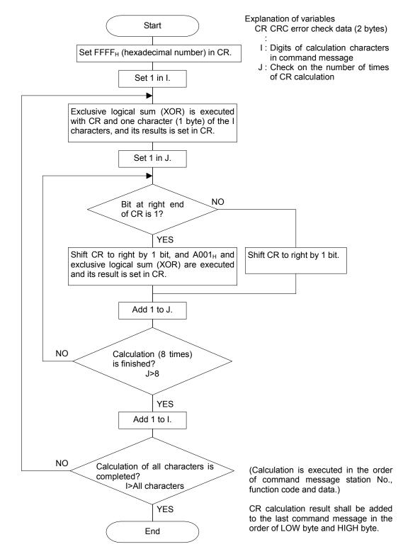
Fig. 5-3 Flow of CRC-16 calculation
