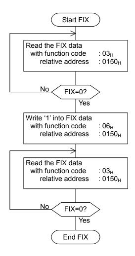
Fig.5-4 FIX procedure
