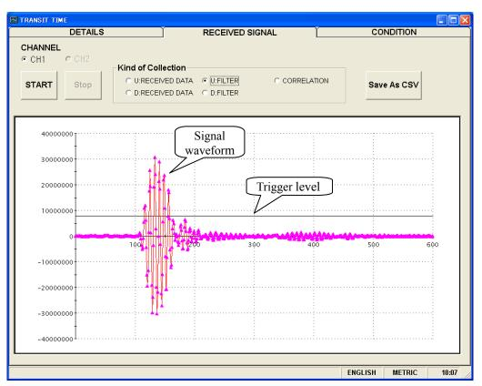
Fig. 9-24 < Received signal screen >
