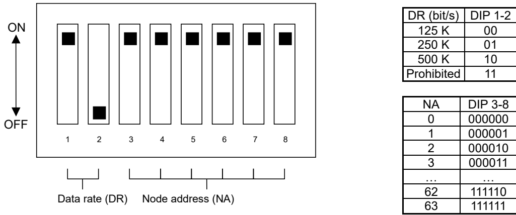
Fig. 11.12-1 DIP switch details (in the diagram, the node address is 63, and the data rate is 500 kbit/s)
